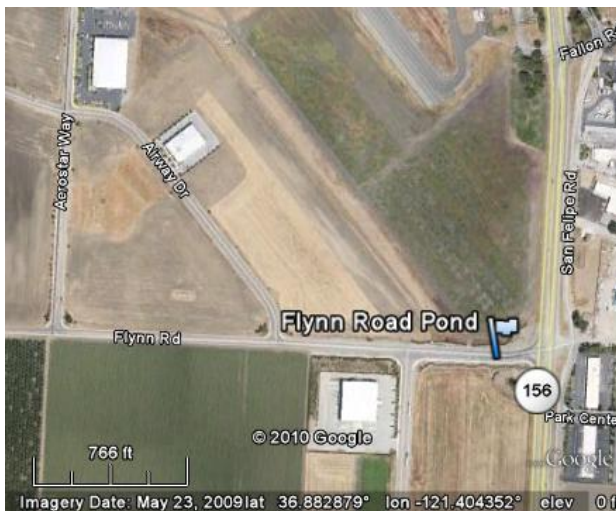
Flooding on north side of Flynn Road near the Flynn Road Pond may be caused by the absence or burial of storm drain inlets to the west at AeroStar Way.
